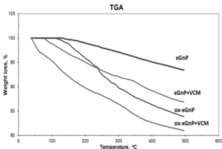
Fig. 3. Comparative thermograms for xGnP and xGnP + VCM, ox-xGnP and ox-xGnP + VCM
