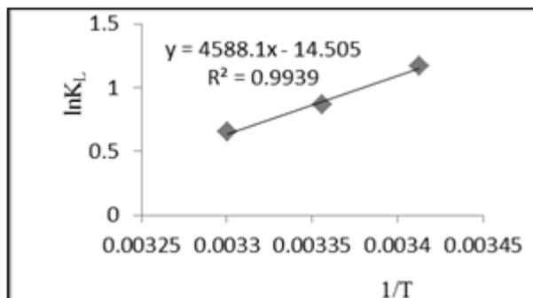
Fig. 9. Thermodynamic parameters of the adsorption of VCM on ox-xGnP in the following conditions:  $pH=7.0$ , temperatures 293 – 303 K, amount of xGnP or ox-xGnP 0.01 mg, volume of solution 10 mL, initial concentration of VCM 25 mg L<sup>-1</sup>.
