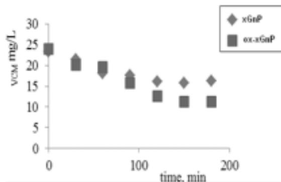
Fig. 4. Effect of the contact time on the adsorption of VCM on xGnP and ox-xGnP. Conditions:  $\text{pH}=7.0$ , temperature  $293\text{ K}$ , initial VCM concentration  $25\text{ mg L}^{-1}$ , amount of xGnP, or ox-xGnP  $0.01\text{ mg}$ , volume of solution  $10\text{ mL}$
