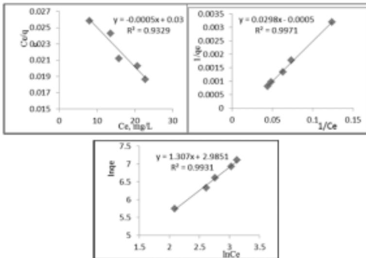
Fig. 6. Adsorption isotherms Langmuir 1, Langmuir 2 and Freundlich of VCM onto xGnP at different initial VCM concentrations. Conditions: pH=7.0, temperature 293 K, amount of xGnP or ox-xGnP 0.01 mg, volume of solution 10 mL.
