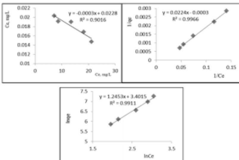
Fig. 7. Adsorption isotherms Langmuir 1, Langmuir 2 and Freundlich of VCM onto ox-xGnP at different initial VCM concentrations. Conditions: pH=7.0, temperature 293 K, amount of xGnP or ox-xGnP 0.01 mg, volume of solution 10 mL.
