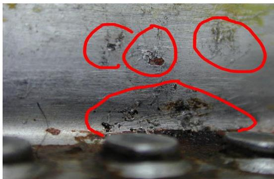
Fig. 3 Corrosion points on the surface of the tank
