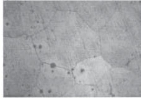
Fig. 1d  $\text{Ni}_{50}\text{Mn}_{25}(\text{Ga}_{12.5}\text{Al}_{12.5})$  alloy (as cast)
