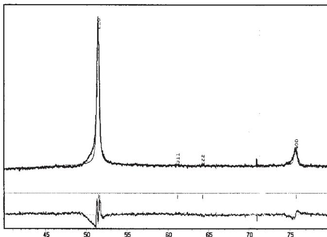
Fig. 4. Diffractogram of as cast Ni<sub>50</sub>Mn<sub>25</sub>Ga<sub>25</sub> alloy (observed data-black; calculated-red; difference-green)
