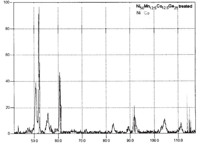
Fig. 2b Possible (Ni)/(Co) solid solutions present in the treated  $\text{Ni}_{50}\text{Mn}_{12.5}\text{Co}_{12.5}\text{Ga}_{25}$  alloy
