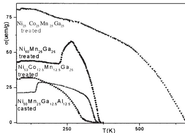
Fig. 5 Variation of specific magnetization with the temperature and nominal composition for treated/as cast alloys
