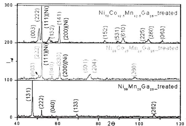
Fig. 3b Diffractograms of treated alloys
