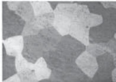
Fig. 1b (Ni<sub>25</sub>Co<sub>25</sub>)Mn<sub>25</sub>Ga<sub>25</sub> alloy (treated)
