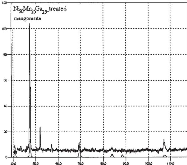
Fig. 2a A small concentration of manganese oxide is present at the surface of the treated  $\text{Ni}_{50}\text{Mn}_{25}\text{Ga}_{25}$  alloy
