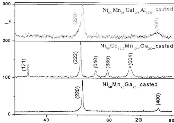
Fig. 3a Diffractograms of as cast alloys
