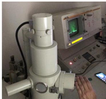
Fig.1. Examination procedure using the scanning electron microscope JEOL - JSM-5200 (Sapientia University of Tirgu Mures)
