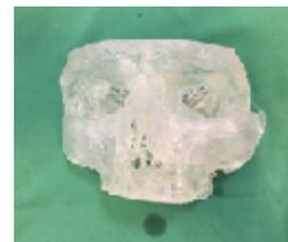
Fig.2 The 3D printed mold used for tailoring the titanium mesh
